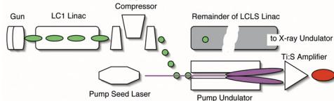
Figure 1: A schematic of the front end of the LCLS with a multibunch beam diverted into a seeded FEL acting as a pump for a Ti:S amplifier.
