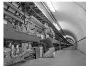
**Fig. 1.2** Bend magnets associated with the Tevatron collider, presently the world's largest highest-energy synchrotron.
