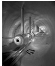
**Fig. 1.1** The interior of an Alvarez drift-tube linear accelerator cavity, showing the drift tubes and their supports.
