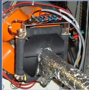
Modified F-line: BPMs (left) and steering coils (bottom).
