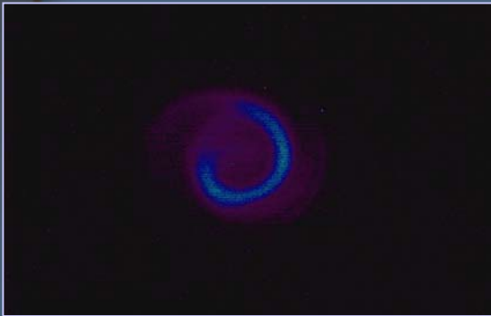
Far Field Angular Distribution patterns for FEL in “low” bandwidth regime
