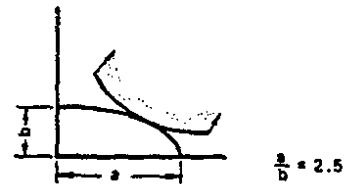
Fig. 3. \frac{1}{4} of aperture ellipse and poleface in original geometry.
